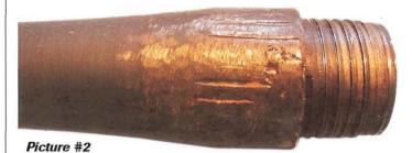
The results when a pipe wrench is used as a barrel removal tool.
