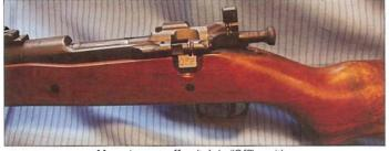
Magazine cut-off switch in "Off" position
